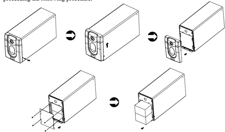
1. Remove the screws on the battery cover.
