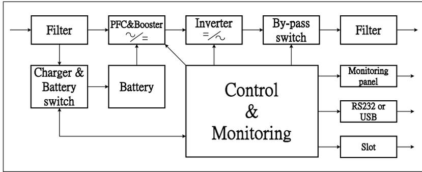
**Fig.1.** Block diagram
